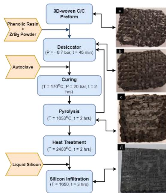
**Fig. 1.** Flow chart for the process of fabricating C/C-SiC-ZrB<sub>2</sub> composites by the combined process of I-CVI, SI and LSI, and Photographs of a) 3DW, b) 3DW + I-CVI, c) 3DW + I-CVI + SI and d) 3DW + I-CVI + SI + LSI preform
