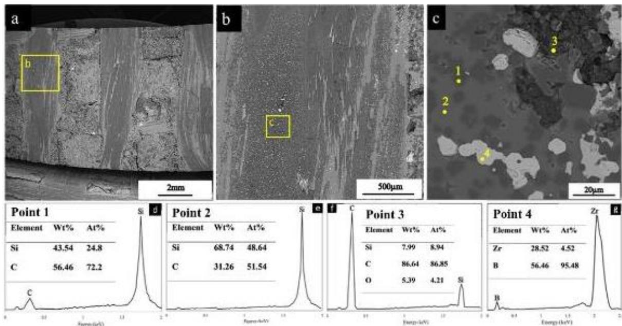
Fig. 5. a-c) Back-scattered electron images of the cross sections of C/C-SiC-ZrB<sub>2</sub> composite, and e-h) EDS analyses of different spots
