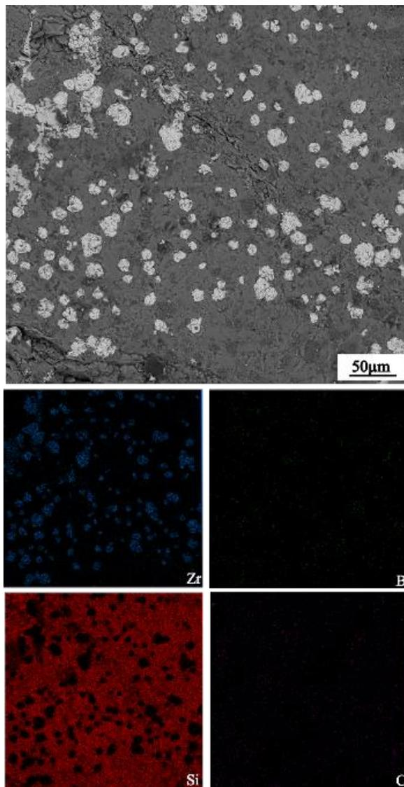
Fig. 6. SEM image and EDS mapping of a representative C/C–SiC–ZrB<sub>2</sub> composite area
