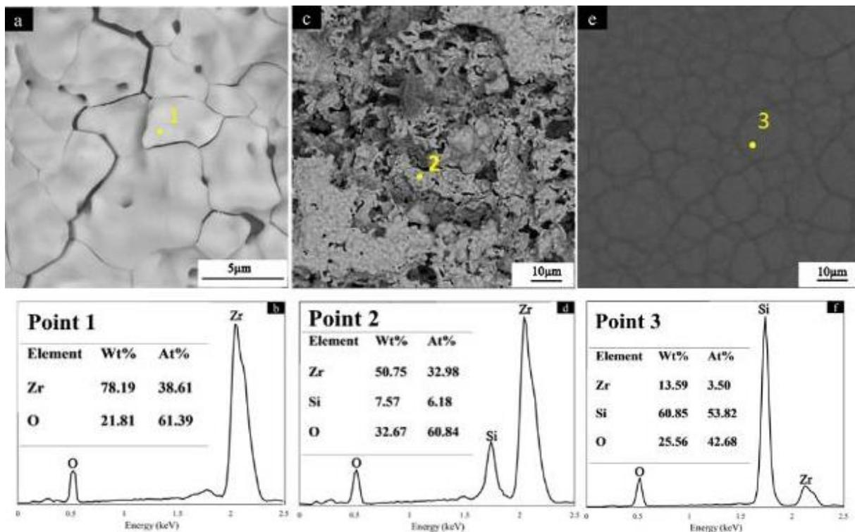
Fig. 11. Back-scattered electron images and EDS analyses of the C/C-SiC-ZrB<sub>2</sub> composite ablated surface in oxyacetylene flame: a) center, b) transition and c) border regions
