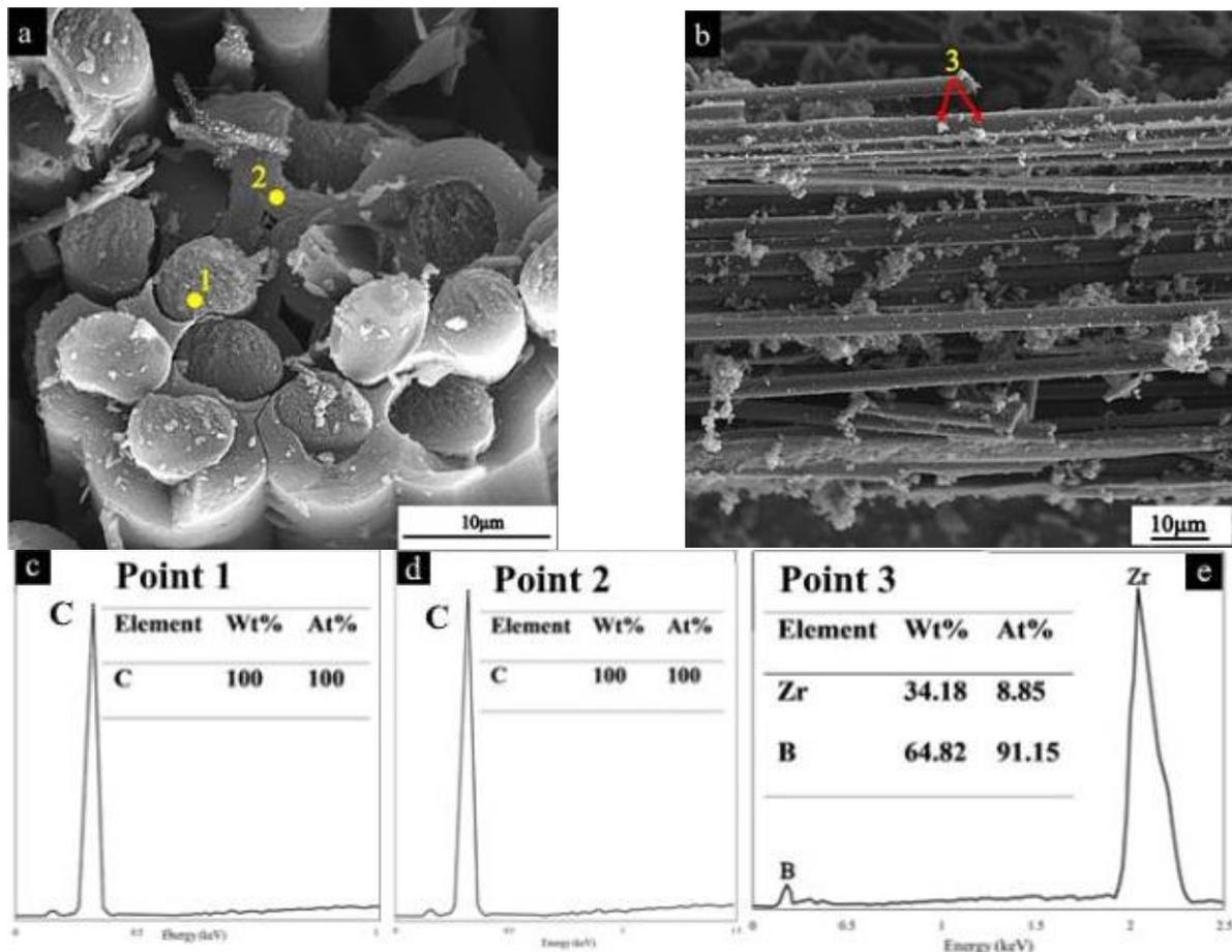
Fig. 3. a and b) SEM images of the microstructure of C/C and C/C–ZrB<sub>2</sub> composites (before the LSI process) and c, d and e) EDS analyses of the indicated points
