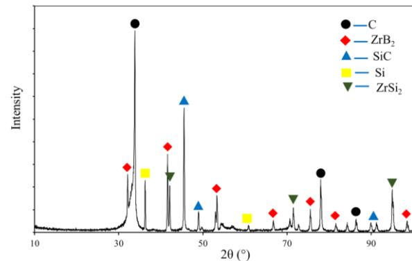
Fig. 7. X-ray diffraction patterns of different C/C–SiC–ZrB<sub>2</sub> composite
