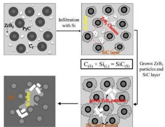
Fig. 8. Depiction of the changes in microstructure and the formation process of C/C–SiC–ZrB<sub>2</sub> composites during the LSI process
