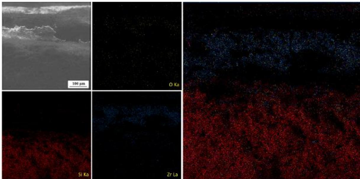
Fig. 14. Elemental map of the cross section of C/C-SiC-ZrB<sub>2</sub> composite after the oxyacetylene torch test
