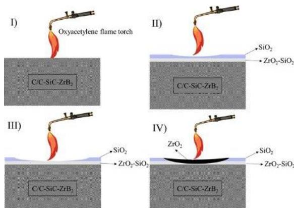
Fig. 15. Surface ablation phenomena of 3DW C/C-SiC-ZrB<sub>2</sub> composite
