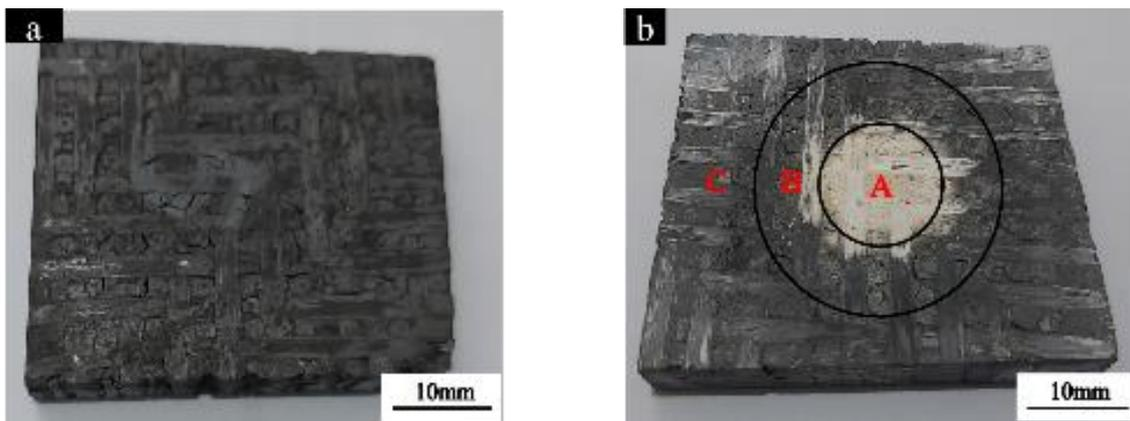
Fig. 9. Macroscopic images of the C/C-SiC-ZrB<sub>2</sub> composite a) before and b) after the oxyacetylene torch test
