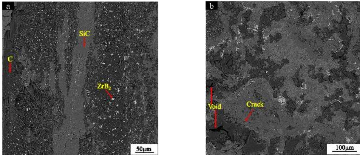
Fig. 4. Cross-sectional microstructures of the C/C-SiC-ZrB<sub>2</sub> composite: a) micro-cracks and b) scattered voids
