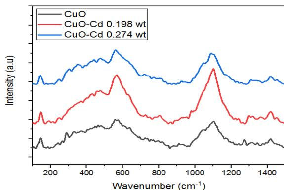
**Fig. 5.** Raman spectra of CuO and CuO:Cd
