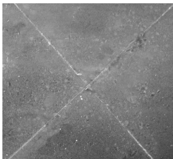
Fig. 5. Surface images of scribed coatings after 1000 hours salt spray test: a) Neat resin b) 3M0T, c) 0M3T, d) 3M3T and e) 3M4T.
