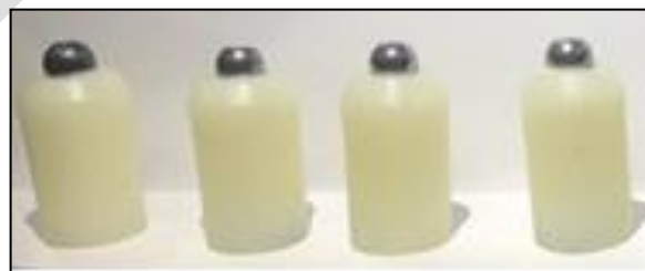
Fig. 3. Photo of the final shape of the bullet used to hit the target object in the gas gun facility
