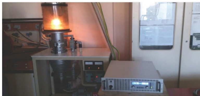
Fig. 1. Working evaporation chamber
