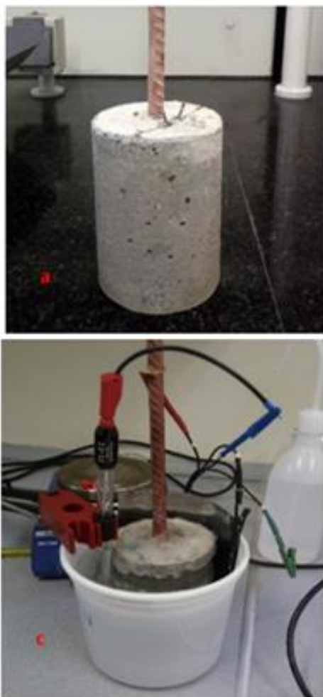
Fig. 7. Concrete sample prepared for EIS (a, b) and test set up for EIS (c, d)
