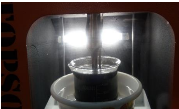
Fig. 6. Sonication devise used to form the GO mix
