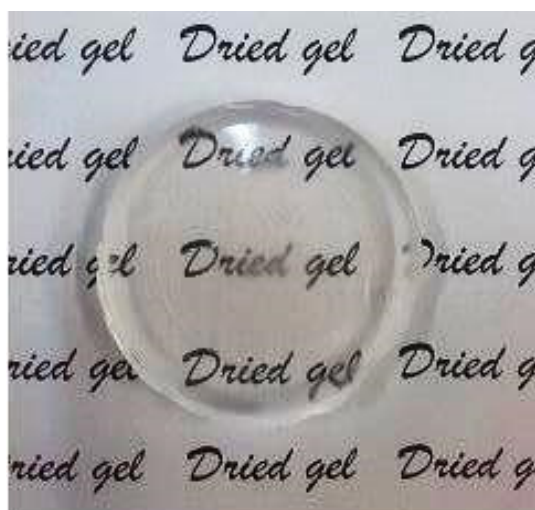
Fig. 2. Monolithic dried gels prepared after 2 month slow drying at room temperature (AD)
