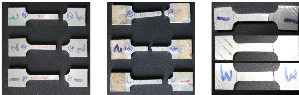
Fig. 9. Tensile tested samples of composites prepared at various pouring temperatures.
