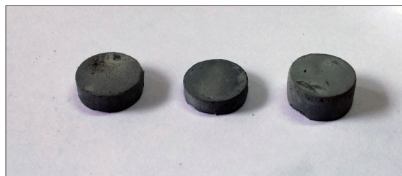
Fig.2. compacted pure silicon after pressing
