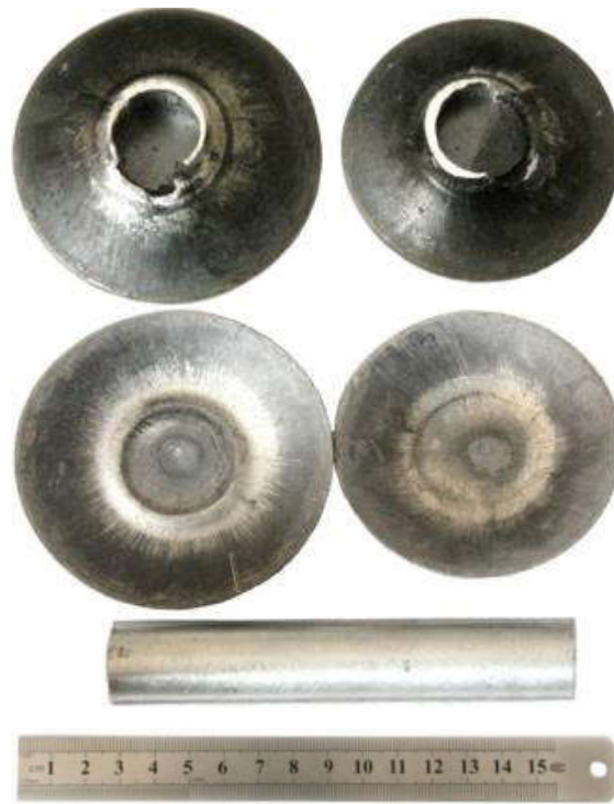
Fig. 2 Initial billet of AM60 and dish-shaped samples fabricated by spread extrusion.
