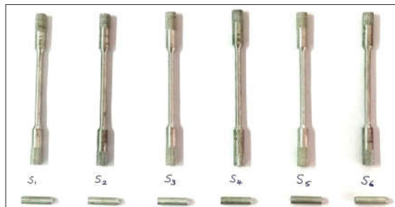
Fig. 3. Tensile and wear test samples
