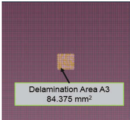
Fig. 3. Top view of delamination incorporated.
