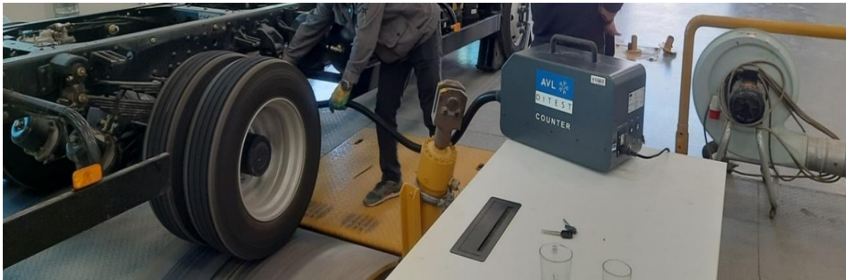
Figure 3: Device for measuring emitted particulate matter
