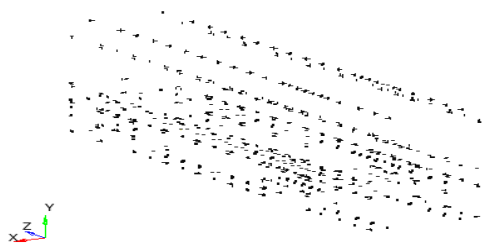
Figure 4: Bus rigid welding RBE2
