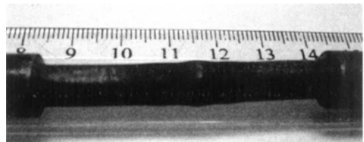
Fig. 9 Flow localization in G4 specimen deformed at 1100 °C and \omega=10 rad/s after applying reheating cycle
